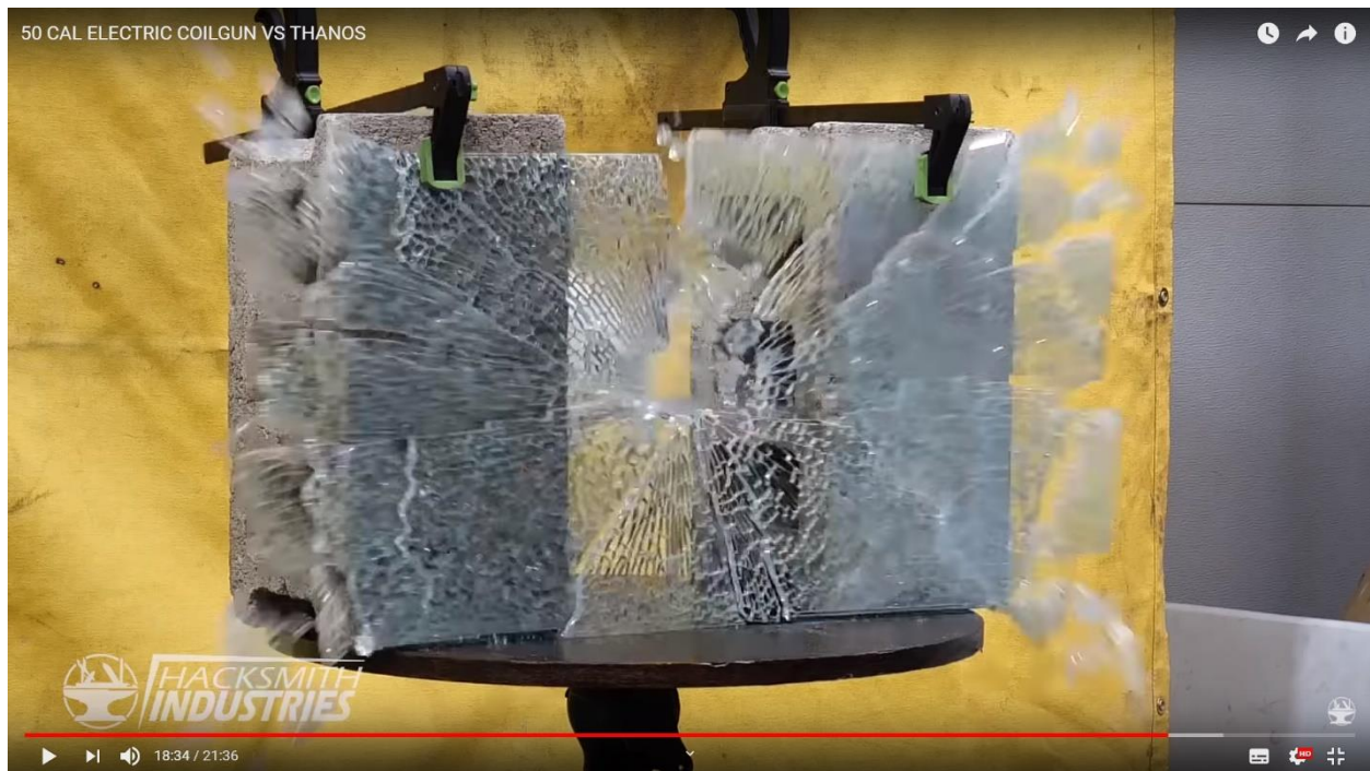
Figure 19 Pane of 3/8" tempered glass shattering and dispersing upon being shot with the coilgun. Copyright Hacksmith Entertainment Ltd. Used with permission.
