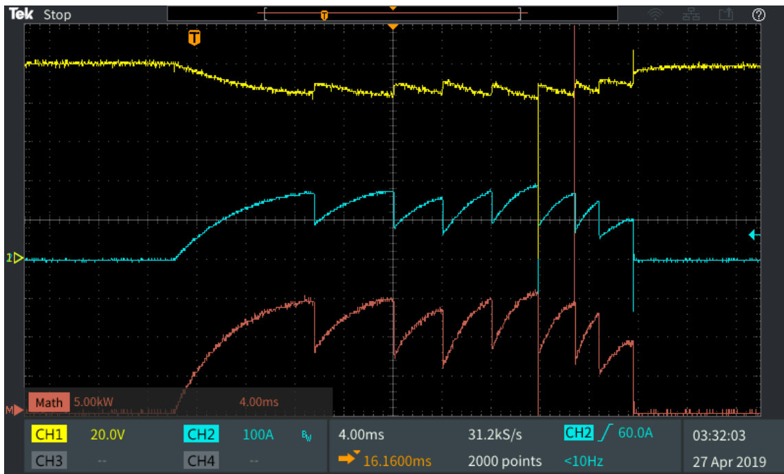
Figure 17 Dual stage tuning. Current, voltage, and power measured through and across battery connections.
